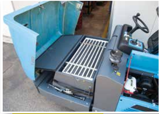
Filtro a sacche in tessuto poliestere con squotifiltro elettrico Dust filter in polyester-textile with electric filter shaker
