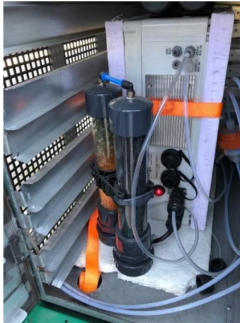
Figure 5.5 – In-situ measurement of the NO 2 adsorption efficiency. Airyx ICAD measurement device installed in a filter column (phase III).
