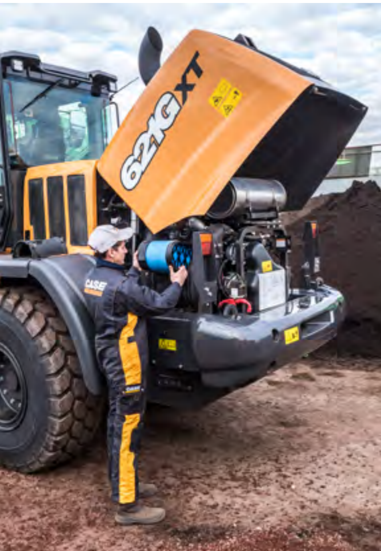
Hood opening and battery on/off switches. In case of flat battery, hood can be opened externally with Remote jump start
