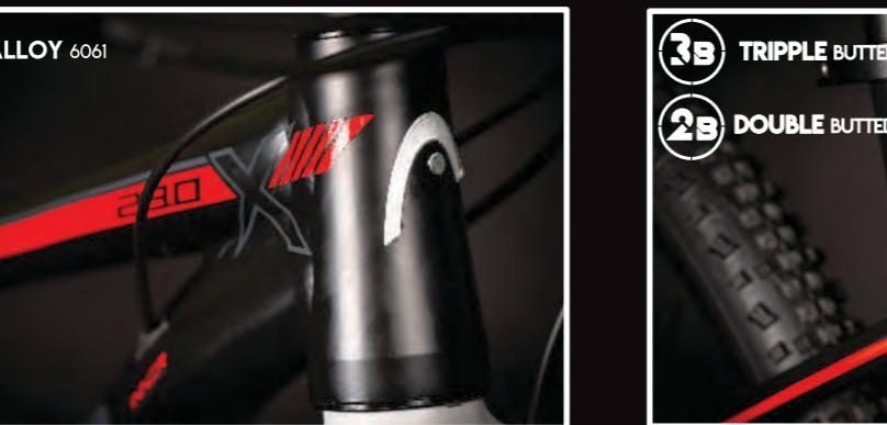
Frames made of 6061 alloy are stiff and resistant to breakages, while retaining the light mass typical for aluminum. They are also heat-treatable after the welding, that also improves frames durability.
