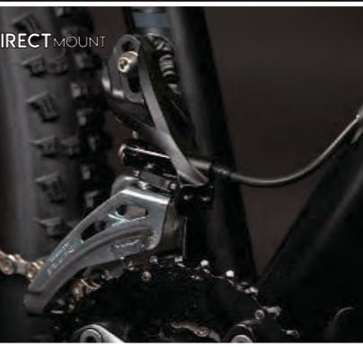
Direct mount of the front derailleur allows us to increase the stability of the connection between the derailleur and the frame.
