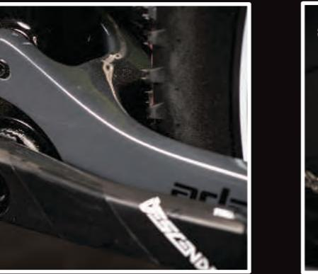
Bearings are placed inside cups and the cups are pressed into the frame to increase pedaling efficiency. These cups reduces bearing wear out and creates a better transfer of the driving force to the wheel.
