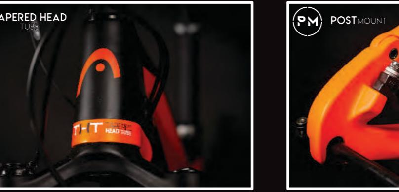
Tapered head tube with increased diameter from 1 1/8" to 1.5" improves the overall stiffness which increases strength of the front of the bicycle. This leads into better precision of the bicycle control.
