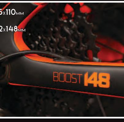
Boost standard hubs - the wider hub flange with 148 mm on the rear hub and 110 mm on the front hub and the stronger spoke-bracing.
