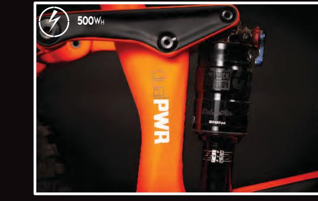
dualPWR - it means combining a classic bicycle with electric drive. We use two variants of motor placing - middle motor and rear hub motor. Drive unit can provide up to 80Nm of torque.
