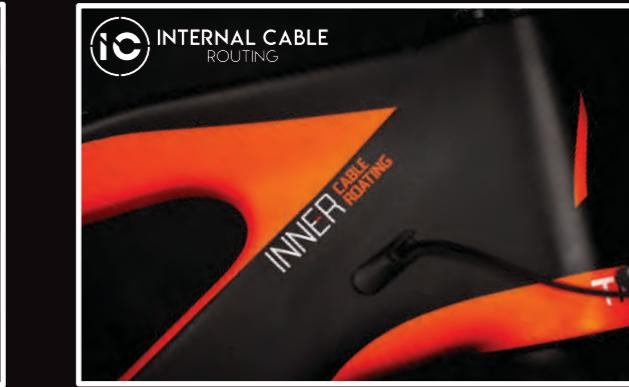
Inner cable routing reduces wear out of cables and shells, it protects them from mud, rain and sand. It also improves the overall appearance of the bike design.
