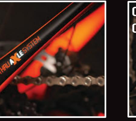
Thru axle system helps us to stiffen the connectivity of the fork and the wheel. The rear thru axle allows us to improve stiffness of the connectivity between the rear wheel and the rear triangle. In overall the thru axle system adds very important stability and precision during the riding.
