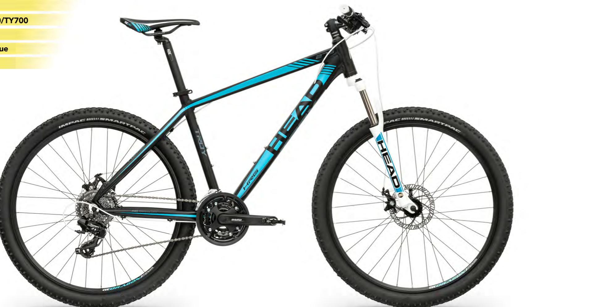
**AL** ALLOY 6061**IC** INTERNAL CABLE ROUTING**PM** POSTMOUNT
