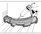
Apply the Effisus Block JP Sealant to the membrane edges. Cover any gaps that may appear.
