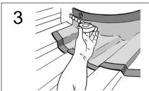
Secure the Effisus Cobra Membrane to the duct by drilling a first screw 50mm from edge for overlap.
