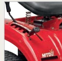
MANUAL CUTTING HEIGHT ADJUSTMENT AND MANUAL PTO
